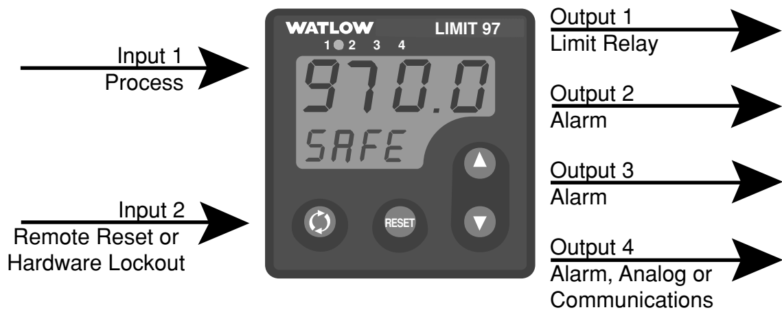
Figure 1.1 — Series 97 inputs and outputs.
