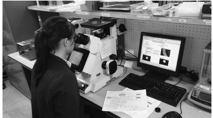
A lab service technician uses a metallurgical microscope to examine the microstructure of the metallic components in Watlow's mineral insulated metal sheathed cable, XACTPAK.
